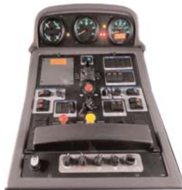
These control panel assemblies for street sweepers were designed 20 years apart using off-the-shelf rocker switches. Today, color LCD displays with touch-sensitive interfaces could replace many of the required controls and dramatically enhance product ease of use.
