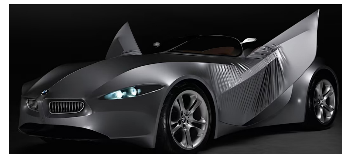
BMW's GINA concept car utilizes a PU-coated Spandex for its skin in place of the usual steel or aluminum. Designers are uniquely positioned to explore these in-context material strategies in ways engineers aren't.
