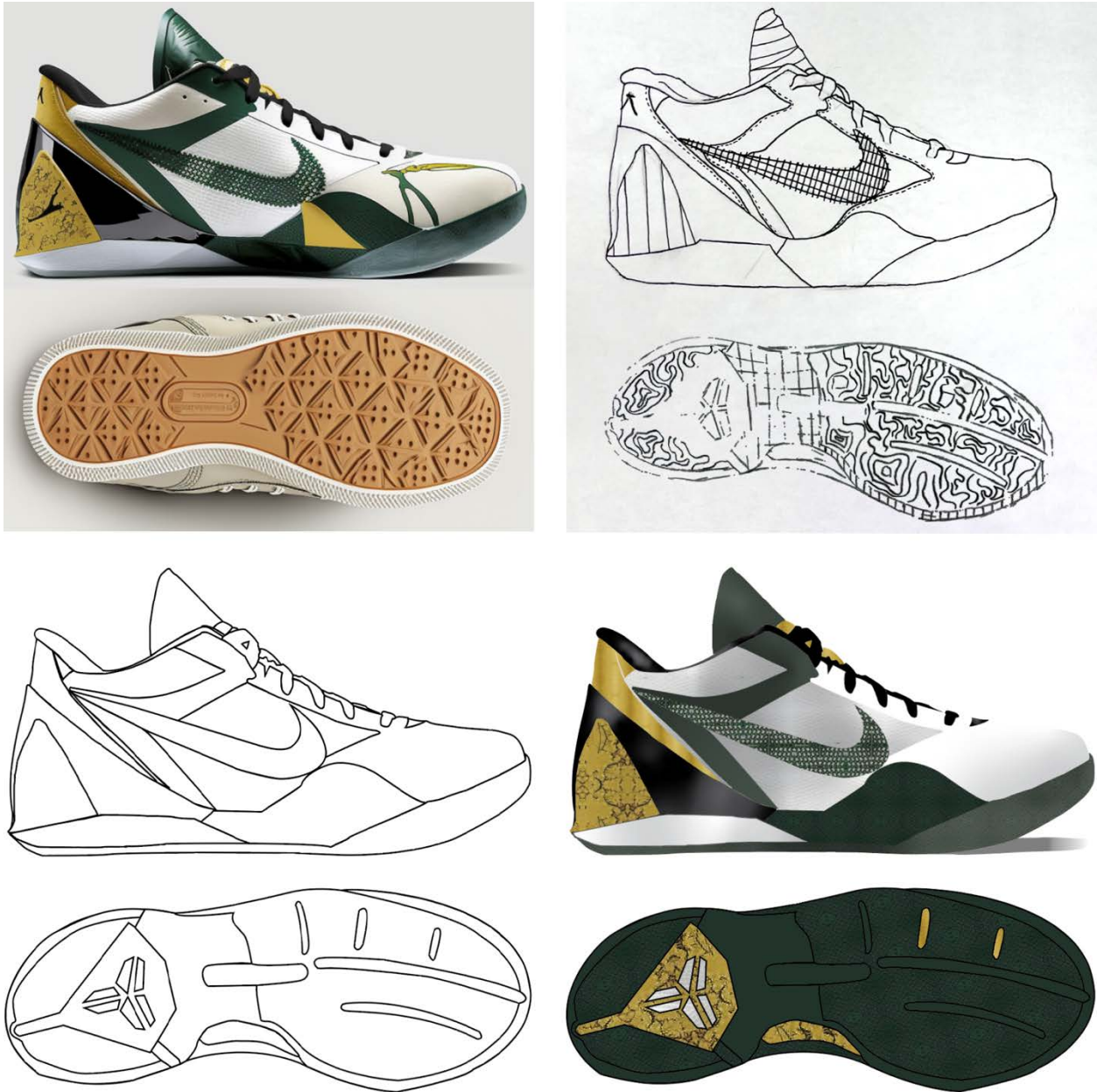
Figure 2. Synthesis of the process followed by students: (1) inspiration images generated in Midjourney; (2) hand-drawn sketches based on inspiration images; (3) outlines of shoe design created in Illustrator; (4) completed shoe design rendered in Photoshop.
