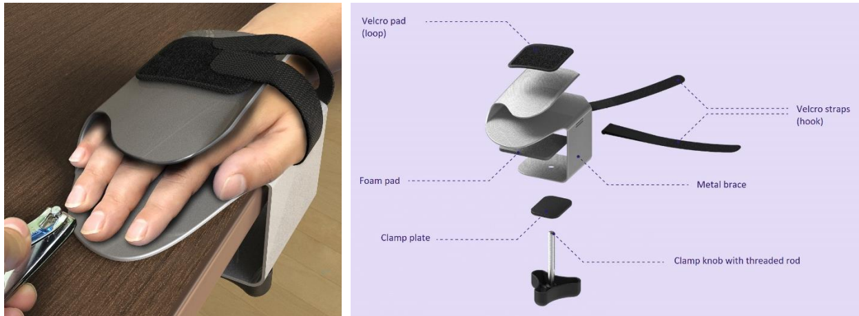
Figure 4. Hold-My-Hand Assistive Brace and exploded view parts diagram. Renderings by Suochun Fang, 2022.
