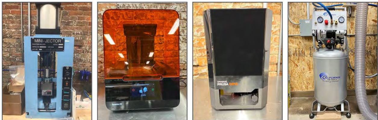
Figure1. From left to right, Mini-Jector Model #45 injection molding machine, Form3 SLA printer, Prusa Curing and Washing Machine and air compressor.
