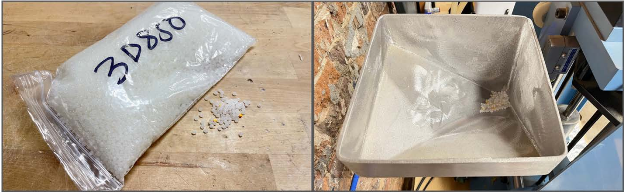
Figure2. NatureWorks 3D850 polylactic acid pellet with yellow colorant and view into the Mini-Jector hopper.
