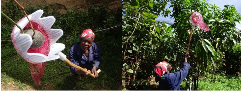
Figure 4. Fruit picker prototype testing
