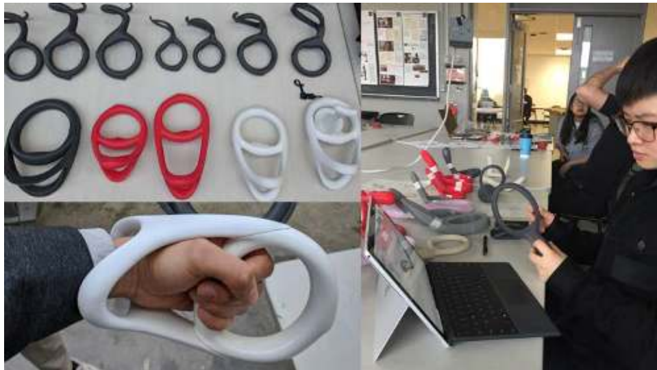
Figure 2: Samples of models from one of the students, including clay, foam, 3D printed, and CAD formats.
