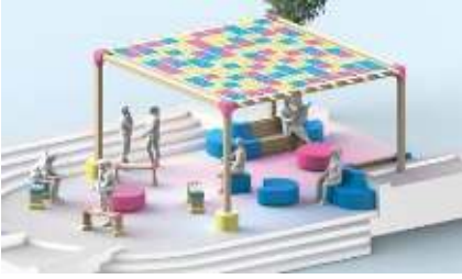
Figure 1. Student parklet concept “Afterhours” proposes the use of modular, 3D-printed components and lumber to form seating and a shade structure in an existing on-campus amphitheater.
