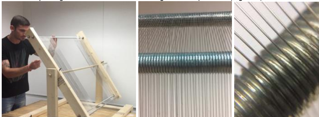
Figure 3: At left, student Josh Tulkoff wiring the first wood harp on a wood spinning frame. At center, a close-up of the stainless-steel wires resting in the threaded rods' grooves. At right, a magnified photograph of the wires resting in the grooves of the threaded rods.
