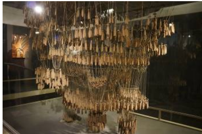
Figure 2. Gaudi’s Hanging Chain Model for La Sagrada Família. Image: KK Clark. http://1.bp.blogspot.com/-IJKiMgirqFU/T7P4wwihD9I/AAAAAAAAApc/B1CmkBIS86U/s1600/DSC00764.JPG
