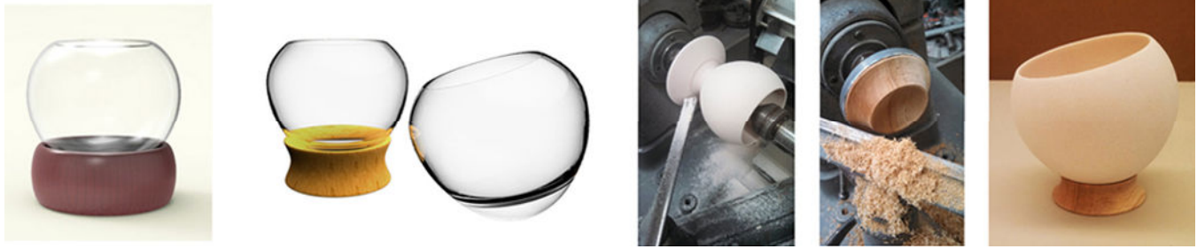
Figure 4: Drinking glass by Timothy Copeland. Development included computer and foam model. Images by: Timothy Copeland.
