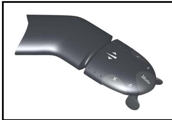
Figure 4. CAID rendering of industrial design proposal as surface geometry only.
